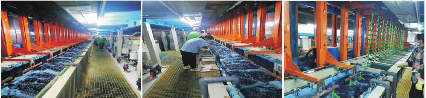
ELECTRO-PLATING LINE, THE MAIN LINE HAS 176 HANGING ARMS, DAILY OUTPUT IS ABOUT 80~100K PCS.
